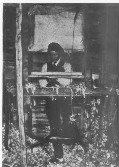
Making a chair: Stages 2 and 3. Top: Young Mr. Dean shaping a LEG with a DRAW-SHAVE. Bottom—Finishing a LEG at the POLE LATHES.
