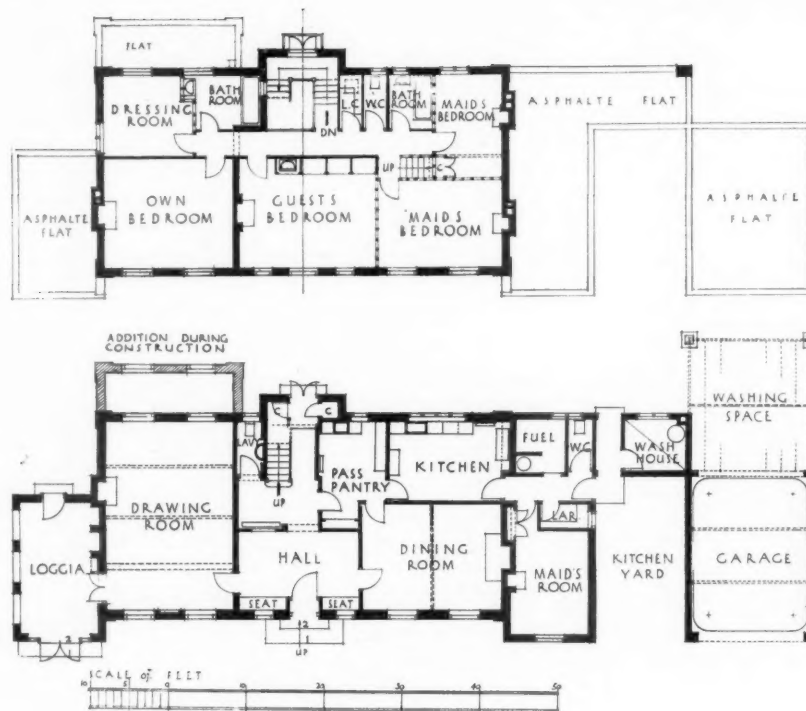
The GROUND- and FIRST-FLOOR Plans.
