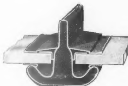
Section of "Eclipse" Patent Glazing Bar.
