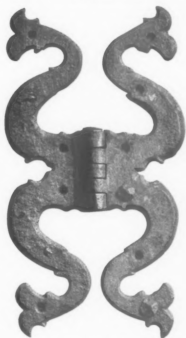
7. H TYPE OF HINGE. The Cock variety, with original nails.
