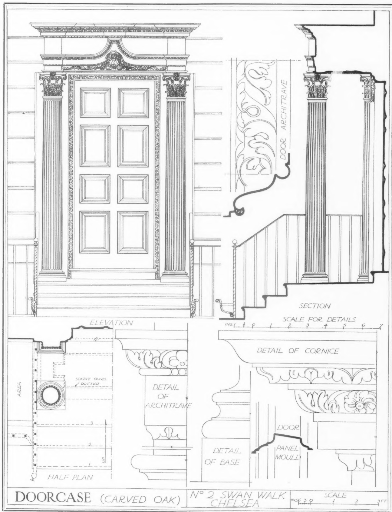
THE FRONT DOOR AND DOORCASE, NO. 2 SWAN WALK, CHELSEA, LONDON.
