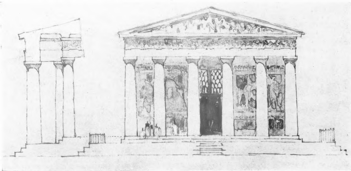
SECTION SHOWING THE RELATION OF THE TWO ORDERS AND THE POSITION OF THE FRIEZE, AND FRONT ELEVATION OF THE PARTHENON AS A PROSTYLE HEXASTYLE TEMPLE.
