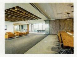
Frameless operable glass walls, like the ones shown here, provide open, flexible integration of spaces when open and private, acoustically controlled spaces when closed.
