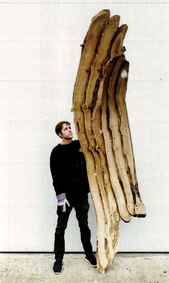
THE WOOD COMPONENTS of Ashen Cabin have been designed to take advantage of the irregular geometries typical of ash trees, including forks and bends.
