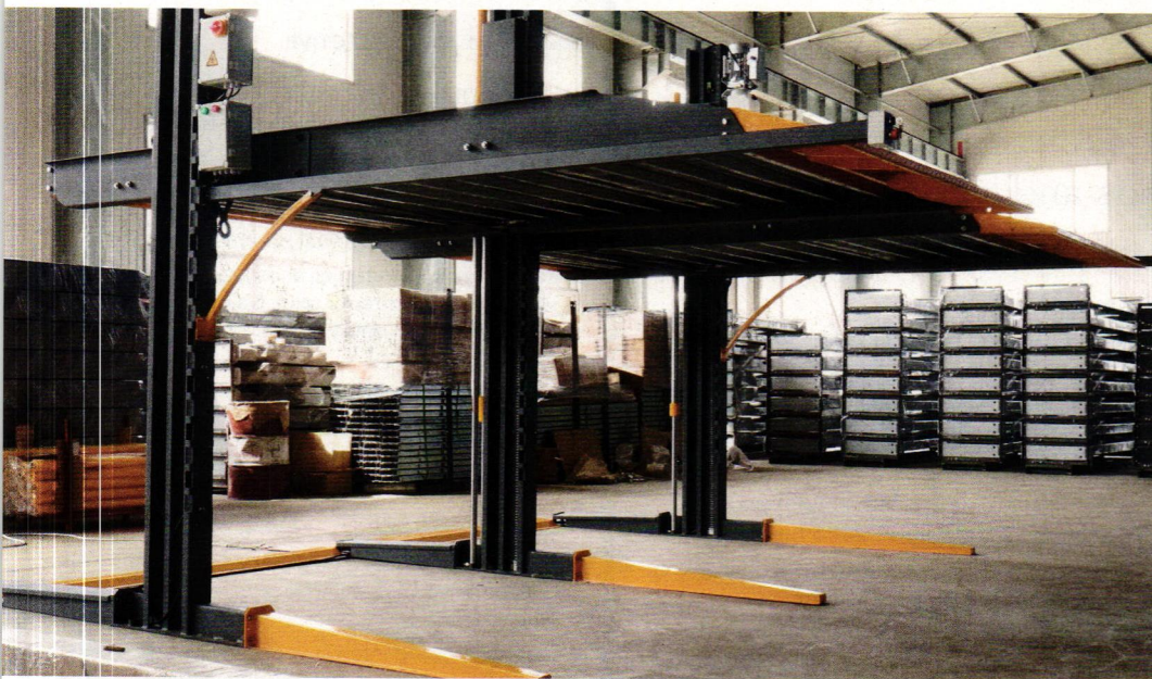
This manually operated parking lift increases the parking capacity of a valet parking area, allowing access to a second-story tier.
