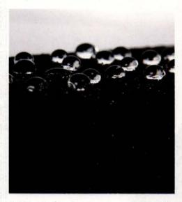
Cellular glass insulation is vapor impermeable, watertight, and can be used to create an additional layer of moisture protection in mission-critical roofs.
