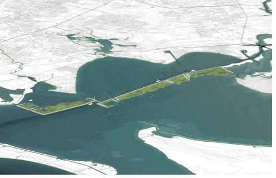
HYBRID SOLUTION Rogers Partners Architects and collaborators propose combining hard and soft flood protections for Galveston Bay that would include floodgates and new parkland, created from soils dredged from a shipping channel.
