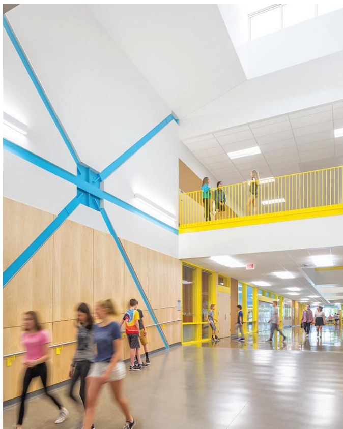
BRACED FOR CHANGE The buckling-restrained braced frame structure (left) at the Mahlum-designed middle school for Oregon's Beaverton School District should enhance its seismic performance. The commons (above) has a backup power supply so that it can serve as an emergency shelter for local residents.
