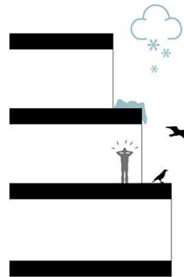
3. VERTICAL FACADE but accumulates snow/ice and bird droppings
