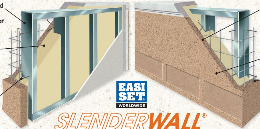
30 lbs. per sq. ft. composite panels, containing 2 inches of precast concrete, are **significantly lighter** than traditional systems, allowing for **larger panels and lower structural and foundation costs**
