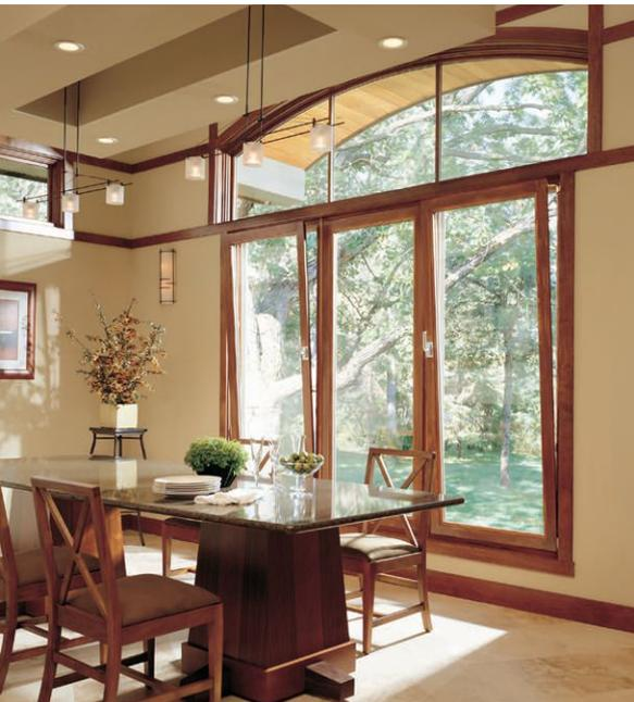
The type and function of operable windows can affect their energy performance, particularly in terms of air infiltration. The tilt-and-turn type shown here, which offers opening options, is generally the most energy-efficient type available from some manufacturers.
