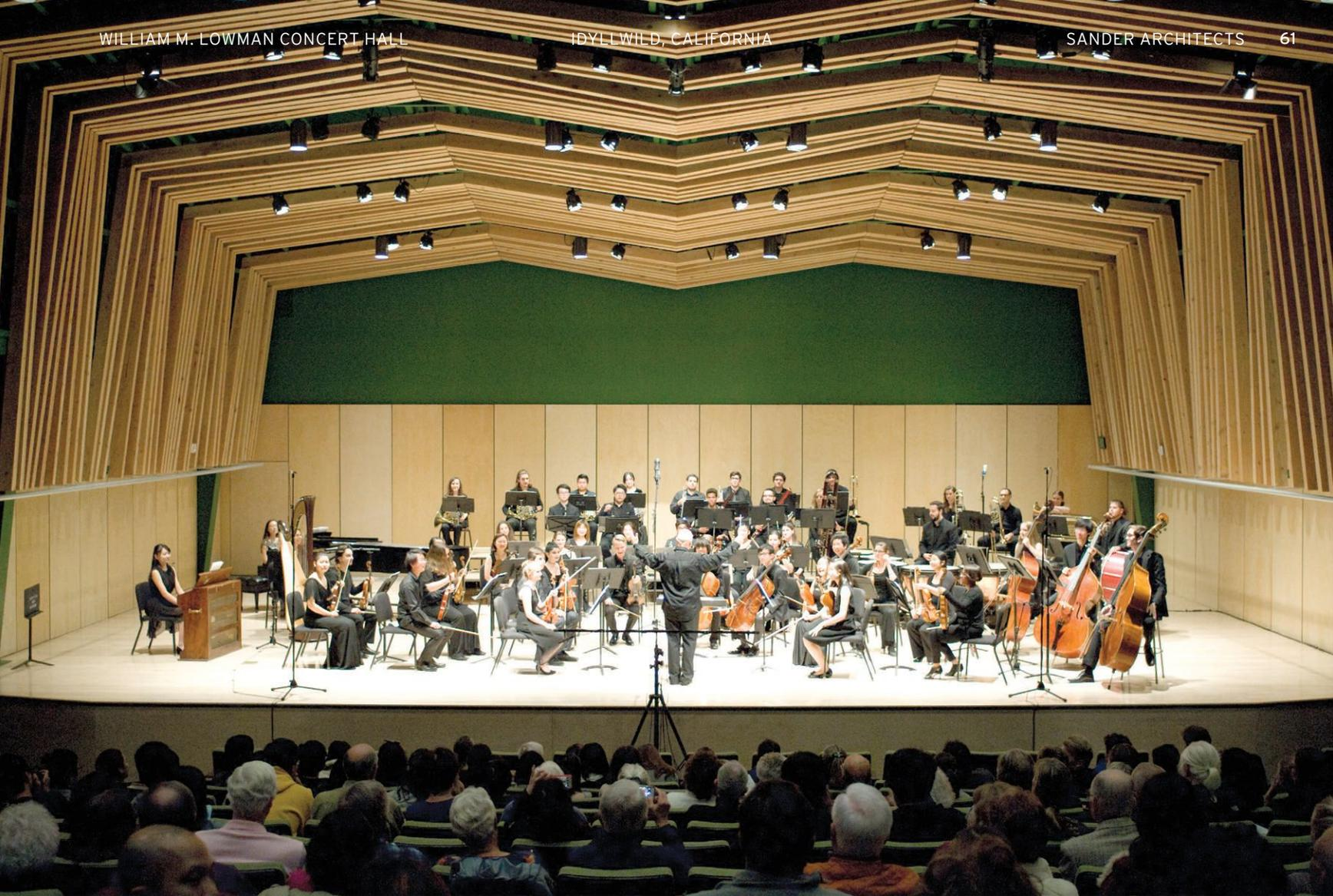
**FINE TUNED** In the plywood-clad lobby, 40 pendant globe lamps hang at various levels (opposite, left). The 4-by-8-inch wood ribs that arch up the side walls and across the ceilings of the performance space are slightly offset to evoke a forest of trees and to scatter the sound and create cleaner acoustics for the performers (opposite, right, and above).
