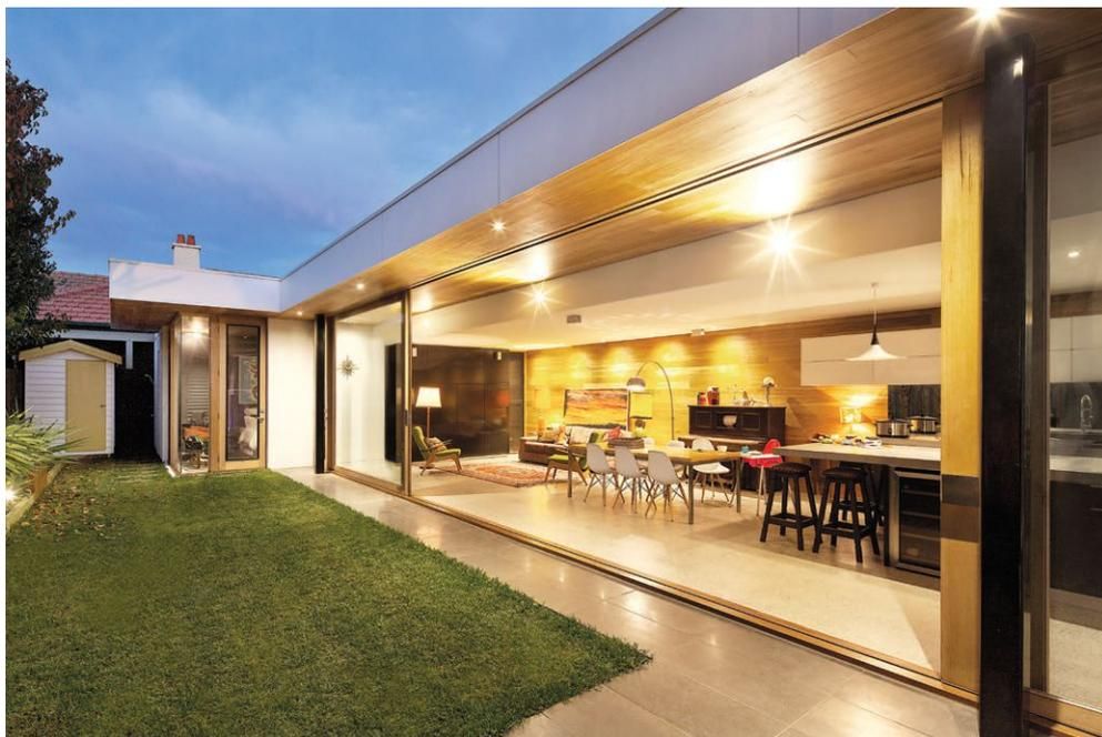
Pictured is an aluminum wood multi-slide system with a stacked configuration with all panels to one side when fully opened.
