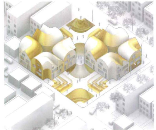
Bair's design for a residential block, as outlined in Cut/Fill , creates multiple corner-lot conditions and reorganizes building adjacencies.
