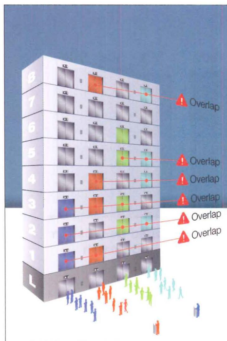
Elevators in conventional destination systems, which may have four stops per elevator, assign passengers with the same destination to the same elevator, but may overlap stops.
