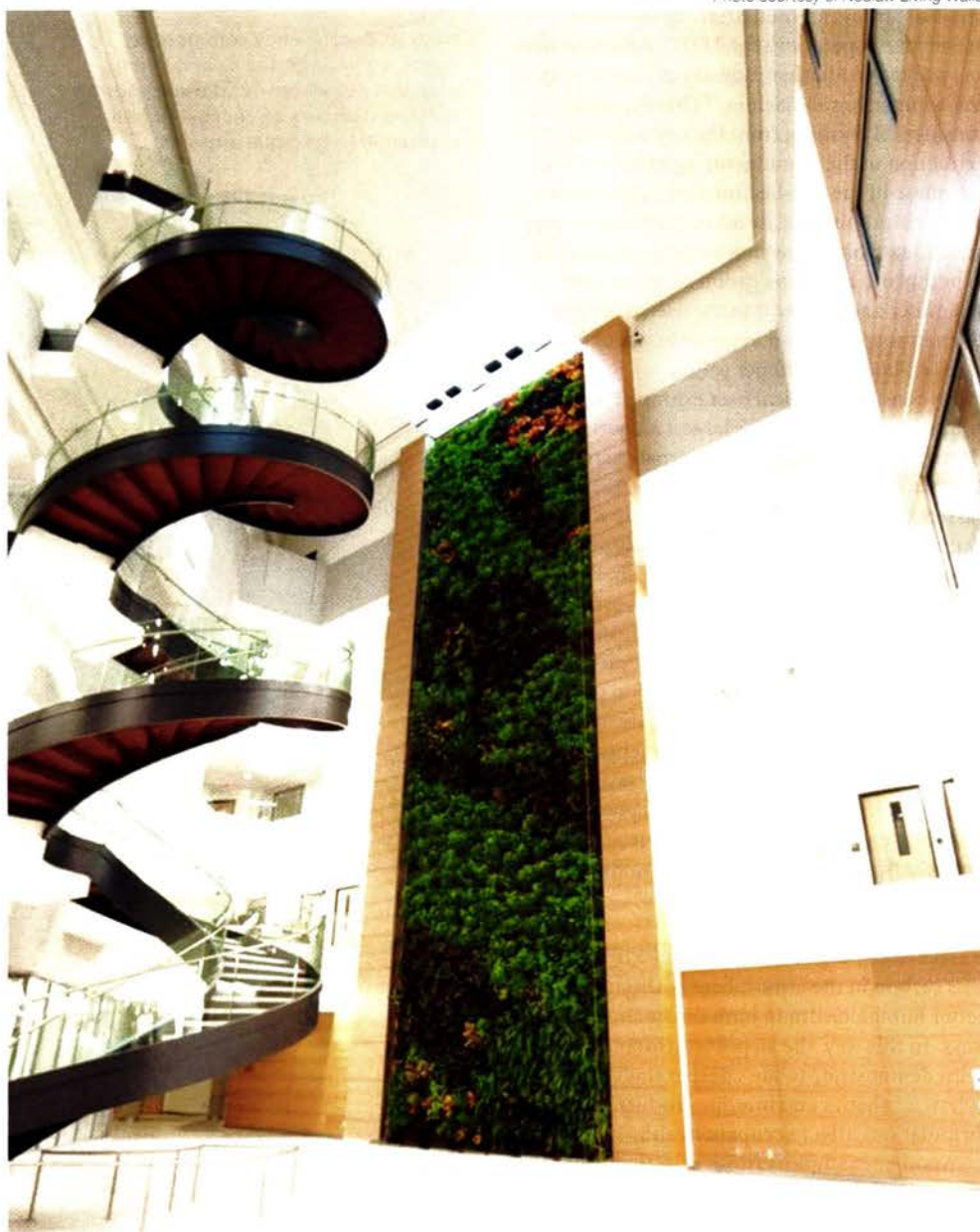
The five-story living wall at Drexel University's Papadakis Building in Philadelphia, designed by Diamond and Schmitt Architects and Nedlaw Living Walls Inc., is the largest of its kind in the U.S. With 1,500 plants integrated into the building's air handling, the system achieves an 80 percent air quality improvement and 30 percent reduction in energy consumption.
