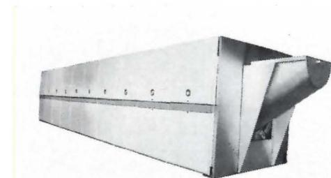
**LAUNDRY EQUIPMENT** / A modular system based on 100-lb washing units, *Milnor's* continuous batch washer for large laundries offers substantial savings in labor, water and fuel. A built-in reuse system saves water and heat; the washer adapts to a variety of floor plans and requires a ceiling height of only 10 ft. ■ Pellerin Milnor Corp., Kenner, La.
