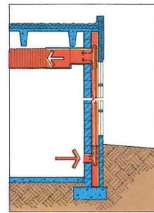
• *Cross section of the modified Trombe wall:* Sunlight passing through windowed wall heats stainless-steel collector plate. Ductwork above brings heated air back into building.
