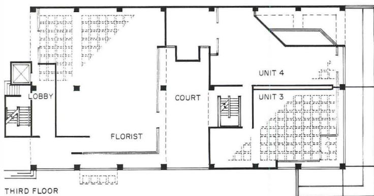
The long-span techniques produced two bays on each floor. The square shape of these bays made the waffle slab—which distributes its loads in two directions—an efficient floor system. It also provides virtually column-free space so that each owner had more than the ordinary degree of
