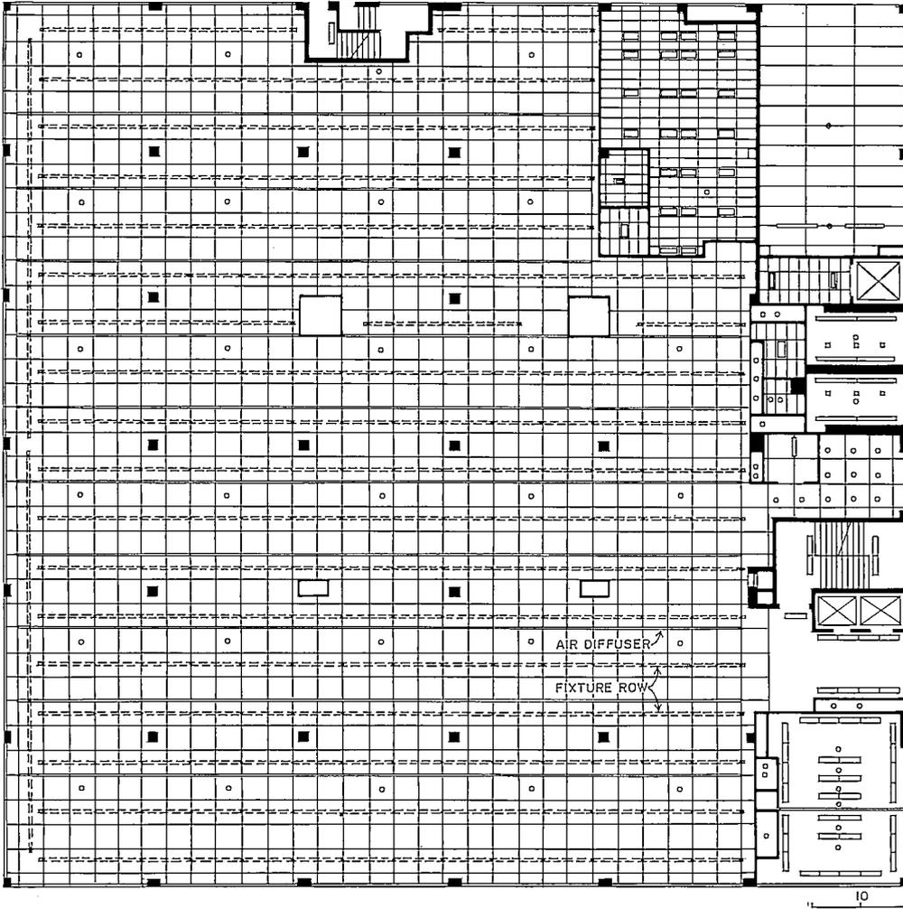
The 10-ft spacing of rows of fixtures corresponds to the 5-ft module of the 1½-in.-thick acoustical ceiling panels, which have high sound absorbency and a light reflectance of 75 per cent. An additional row of cube fixtures near the wall opposite the core illuminates the wall to minimize brightness contrast during the day and to light the
