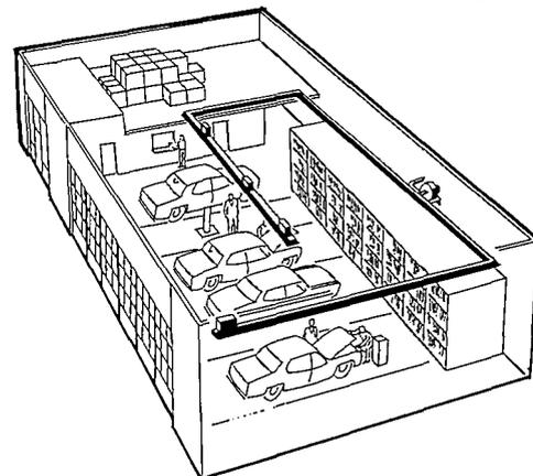
Developed in 1963, Co-Ray-Vac is a fully vented, low intensity infrared heating system. It is used primarily for new or retrofit installations in industrial or commercial buildings.
