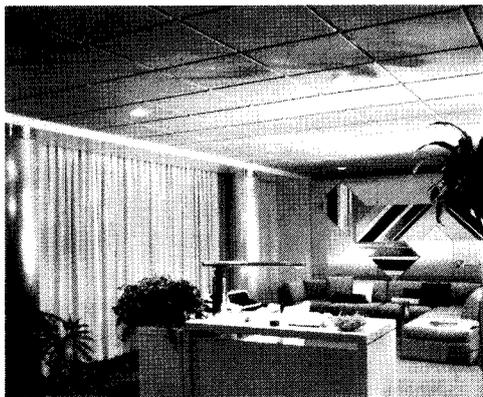
**ACOUSTICAL CEILING** / Recommended for commercial and office applications, fire resistant "Soft Look" ceiling panels have a non-glare fabric surface over a mineral fiberboard substrate. The 2- by 2-ft panels have regular edges for design interest, and to facilitate installation and removal. The porous modacrylic fabric covering is offered in six natural and six accent colors; the exposed grid is also available in various colors and finishes. ■ Armstrong Cork Co., Lancaster, Pa.
