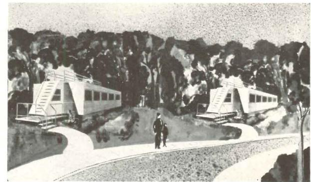
Architect Alfred Clauss of Knoxville, Tenn., offers the above scheme as one possible solution to defense housing needs. Necessary reductions in reproducing his drawings have obscured some details, but we hope not the essential idea. Size of shipping unit, according to Mr. Clauss, is 8 by 9 by 28 ft.; size of extended house, 22 by 11 by 28 ft.; estimated cost, \$900; weight, 6800 lbs.; erection time, one hour, with unskilled labor.
