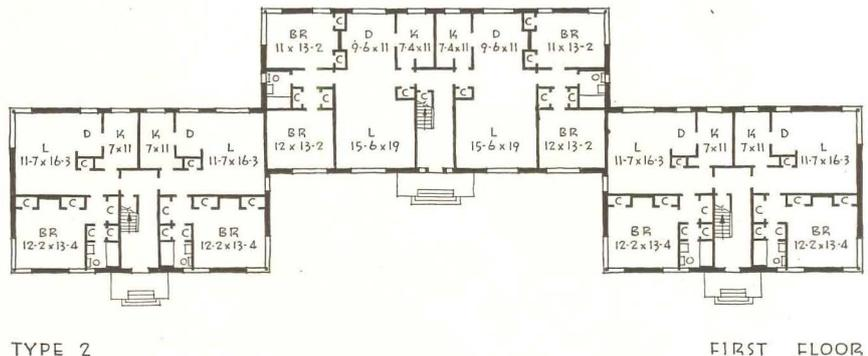
THE PARKLANE Apartments are of brick-veneer construction with specially constructed steel frame and concrete floor slabs. The frame is sheathed with sheathing wallboard and faced with rusty-pink brick and warm gray-white stucco. Fenestration consists of both steel casements and glass-block panels. The roof is of galvanized iron, 29 gauge, with standing seams and covered with four-coat asphalt and sand treatment with a white cement-base finish coat.
