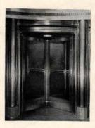
Automatically collapsible and panic proof revolving doors are shown in the catalog of General Bronze Corporation. Doors are available in bronze, aluminum, nickel silver, stainless steel or wood. Free rotation of the revolving wings up to any predetermined rate of speed is made possible by a speed regulator. Elimination of drafts, noise and
