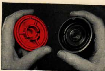
Wheel nut holds black hub on spindle . . . then colored cover snaps on.
