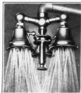
K-3416—SPEAKMAN Anystream Self-Cleaning Unit Control Triple-Cluster Shower Head with 1" I. P. female inlet (patented). For use where a large amount of water is desired. Because of the large size of the head it should be braced to the ceiling.
