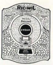
Cross section of Ric-WiL Type F Conduit with DrypaC filler, single pipe installation. Note Base Drain carries the entire weight of pipe supports and pipe independent of the Conduit.
