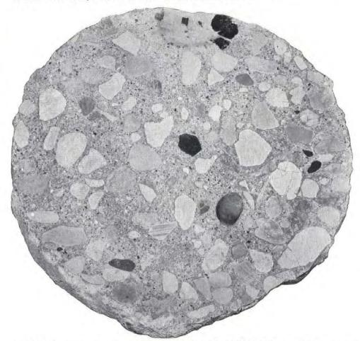
GOOD concrete, compressed by the MacARTHUR method, insures piles of greater bearing capacity. The rough concrete is intimately bonded with surrounding soil.
