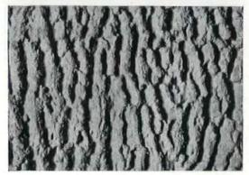
Texture" in Northwestern Terra Cotta nomenclature, is defined as the treatment of the clay surface, before the application of color or glaze, so as to produce any desired pattern, either regular or irregular. The accompanying illustrations indicate a few of possible textures, ranging from the lowest relief to rugged or modeled surfaces.
