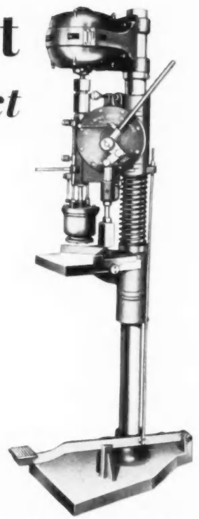
The above—Evans ring joint machine Model M, electrically operated—one man control.
