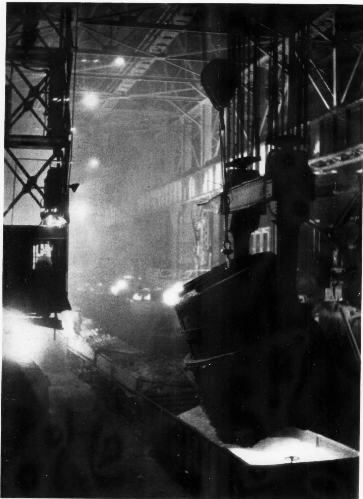
BESSEMER CONVERTER DUMPING A MELT
