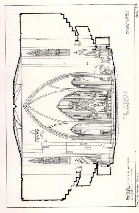
Transverse section of The Miracle setting. The full height of the prosecuium opening is utilized, and no curtain is used. Every effort has been made to bring stage and auditorium into such complete coördination that the spectators shall feel themselves also participators in the spectacle
