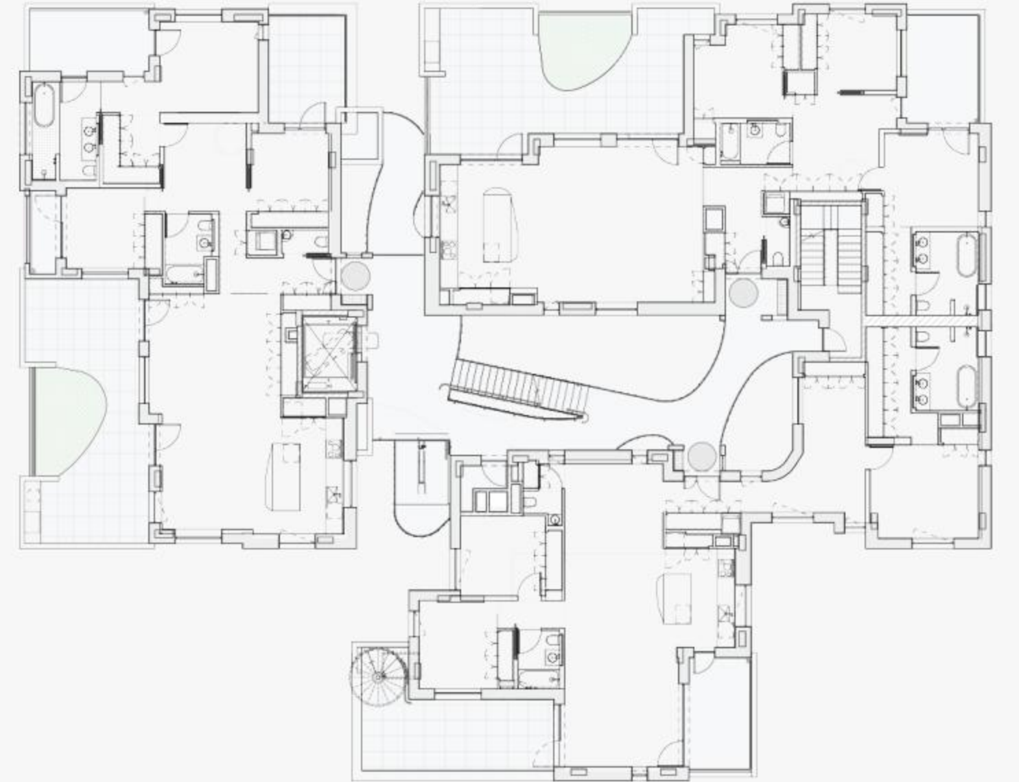
Fifth-floor plan: The three penthouses sport private terraces. The building's three masses, fully separate on lower floors, are joined on the right (eastern) side to connect a primary bedroom suite to its unit.
