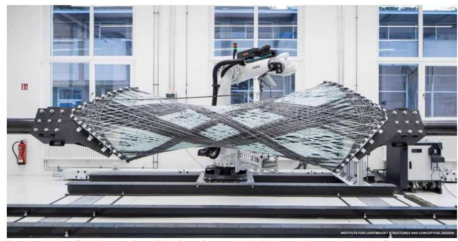
Researchers at the Institute of Building Structures and Structural Design in Stuttgart, Germany, are developing flexible composite fiber structural assemblies for the Elytra pavilion, a domed structure made up of woven glass carbon fibers.
