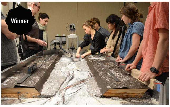
Public Sediment for Alameda Creek is a proposal to address the challenge of sediment scarcity along the vulnerable urban periphery of San Francisco Bay. The initiative aims to redesign the Alameda Creek waterbody and to create a functional system that can sustainably transport sediment and provide a habitat for fish. A physical stream table model was developed to represent a leveed channel condition, and to
