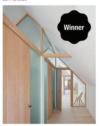
building, linking the newly habitable attic to the levels below. The attic's wood framework is a graphic echo of the original roofline within the expanded building shell. This framework language carries throughout the project in casework details, windows, guardrails, and the kitchen.
