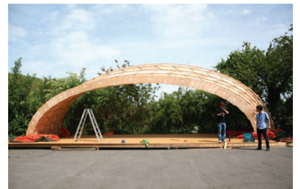
Yves Weinand's work at the IBOIS lab focuses on finding new uses for mass timber, including experiments with long-span structures.
