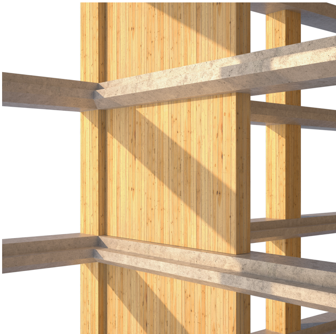
Above and below: SOM's proposal for a 40-story timber tower with a concrete core is based on a structural system designed by Fazlur Kahn in 1965.
