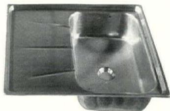
A new Monel sink for motor boats and various industrial purposes has been placed on the market by The Parsons Company, Detroit. It is made in a single piece with an integral drainboard, which can be sheared off if desired. The sink is made of 18-gauge sheet. The complete unit with its drainboard has an overall length of 25 in. and a width of 21 in. The bowl itself is 12 in. by 18 in. by 6 in. The ribbed drainboard and bowl are recessed 7/8 of an inch to prevent water splashing over.
