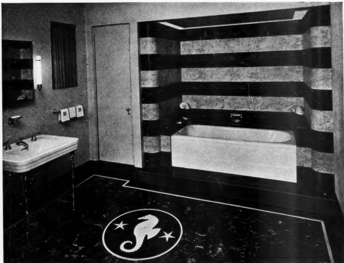
Model bathroom in showrooms of the Crane Co., New York. The floor is a black Sealex Veltone, white veined, with sea horse Linsignia and single line border in ivory. Sealex Wall-Covering, in three marbleized effects, used on all walls and doors.
