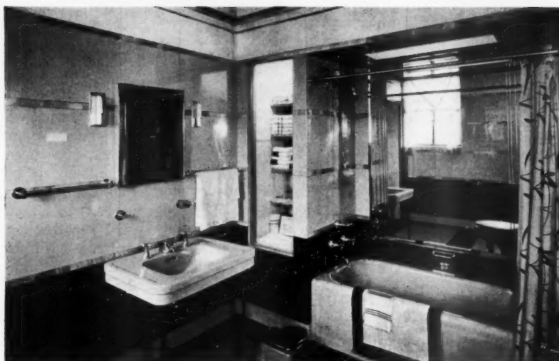
ABOVE: Glass walled bathroom by Paul Nash, London. The various kinds of stippled, clear and reeded glass are alloy-silvered in colors. Floor, pink rubber. RIGHT: Exceptionally well-planned bath in Rostone House, A Century of Progress, Chicago, using ceramic structural slab material for walls. Walter Scholer, architect; Frank Sohn, designer
