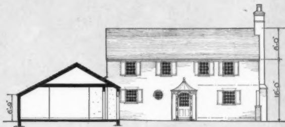
Entrance Side and Section Through Garage
