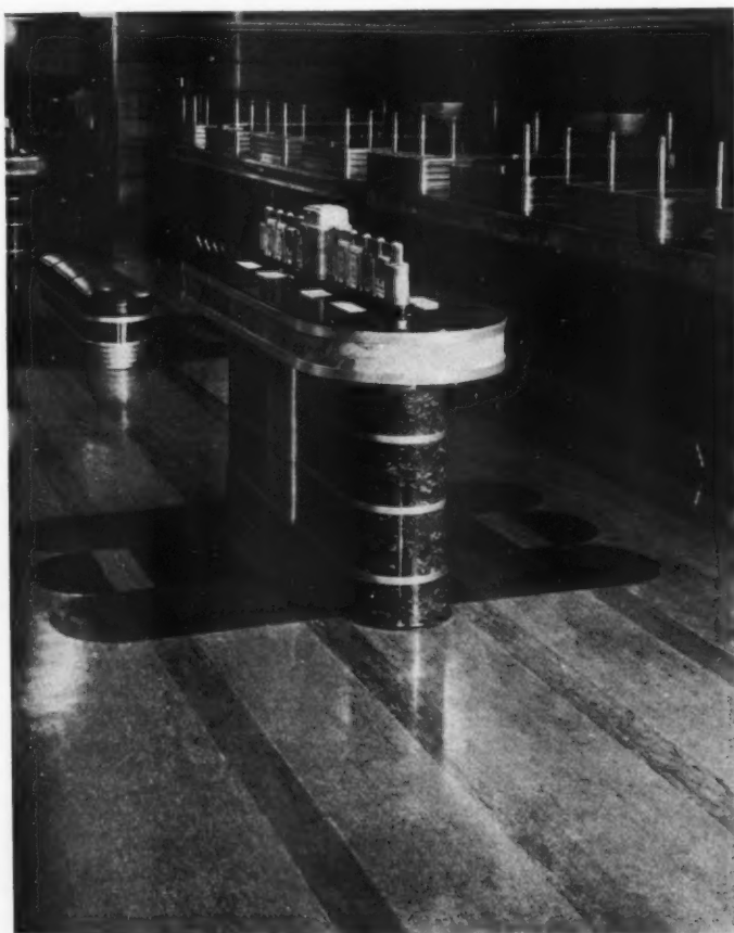
This inlaid compass point of special design is in the Topeka High School, Topeka, Kansas, Jameson W. Williamson & Co., architects. The field is of marbled linoleum laid in segments so that the striations point to the center. Colors used are: 1. Light yellow 2. Light tan 3. Terra cotta red 4. Light blue 5. Chocolate brown 6. Light brown 7. Marbled in gray-brown tones
