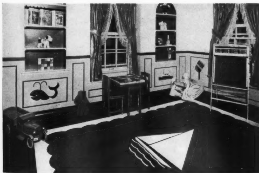
Demonstration nursery in "The Home in the Sky," Cleveland. The floor is of linoleum with a blue center field; white sailboat and border; black outer border and base. The wainscoting is also of linoleum with a white background, blue cap and panel trim, and decorative figures in various colors
