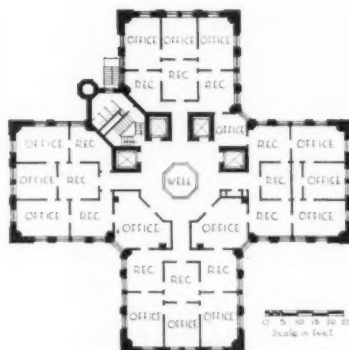
Characteristic floor plan of the 19-story reinforced concrete Medical Arts Building, Dallas, Texas. The dental offices are concentrated on the north side; the ear, nose and throat specialists on the west. The plan offers exceptional light. Note the absence of interior columns in the wings, made possible by the use of long span, two-way, deep joists, which gives maximum flexibility in partition arrangement.
