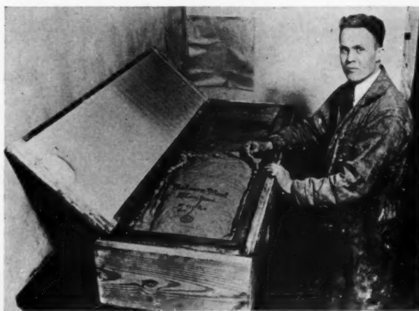
THE TEST: Where insulation is used, lath marks are slight. Where not used, the marks are well defined
