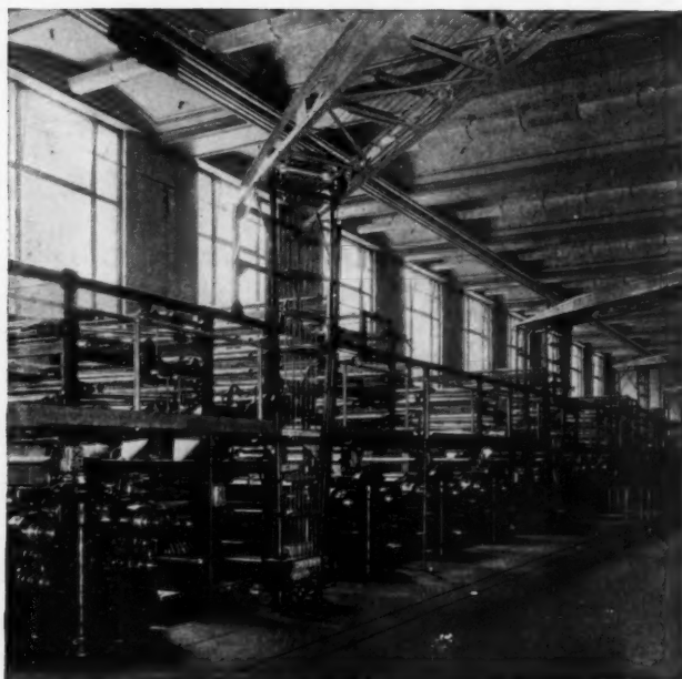
Press room, Brooklyn New York Times Building. Albert Kahn, Architect. Bronze sash by William H. Jackson Co. Presses shown are Wood presses.
