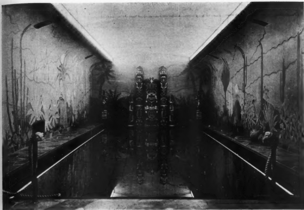
SWIMMING POOL Christian R. Holmes estate, Port Washington, L. I. The tubes are recessed below the water level and protected by a glass facing which need not be water-tight
