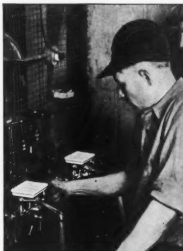
ABOVE—One of the seven major inspections made on each Kohler fitting before it reaches you. Here, the workman is water-testing the casting.
