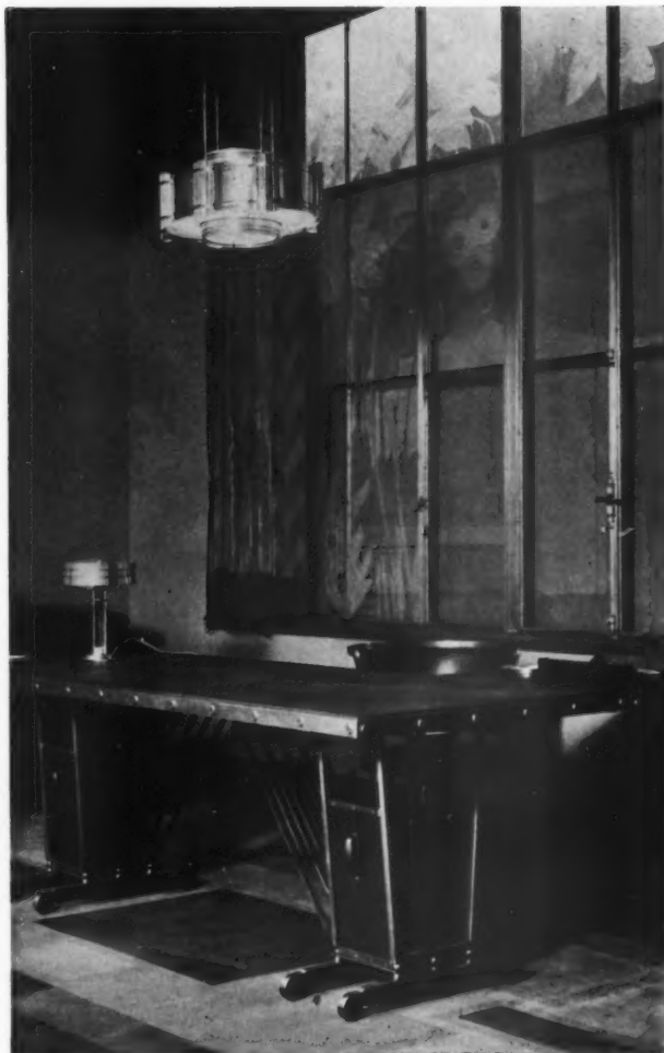
A PENDANT lighting fixture that provides direct and indirect illumination by means of combined high and low intensity lamps
