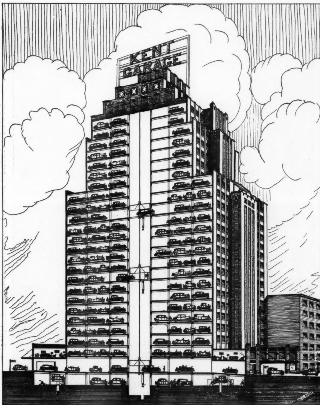
SECTIONAL DRAWING, KENT AUTOMATIC PARKING GARAGE, NEW YORK
