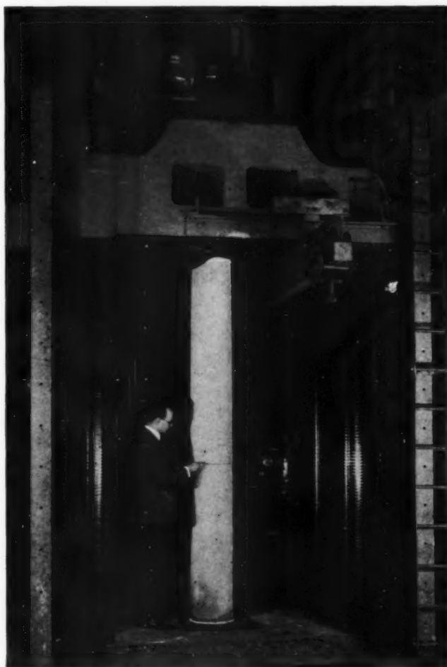
LIMESTONE COLUMN SET UP IN TESTING MACHINE READY FOR LOADING. PLASTER OF PARIS CAPS ARE SEEN AT TOP AND BOTTOM
