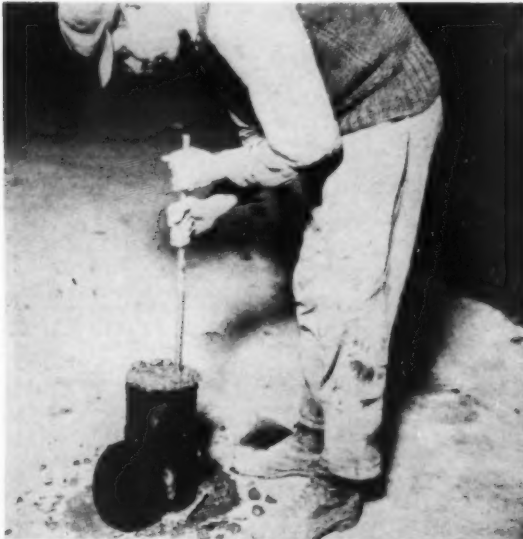
RODDING CONCRETE IN TEST CYLINDER MOLD. CYLINDERS, TO MAKE COMPARATIVE RESULTS OF VALUE, MUST BE CAREFULLY MADE IN THE FIELD AND UNIFORMLY HANDLED AND TREATED IN THE TESTING LABORATORY
