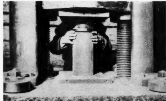
RODDING CONCRETE IN TEST CYLINDER MOLD. CYLINDERS, TO MAKE COMPARATIVE RESULTS OF VALUE, MUST BE CAREFULLY MADE IN THE FIELD AND UNIFORMLY HANDLED AND TREATED IN THE TESTING LABORATORY
