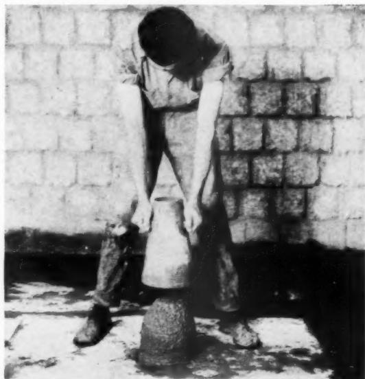
WITHDRAWING THE SLUMP CONE. THE SLUMP TEST IS A SIMPLE METHOD OF REGULATING THE CONSISTENCY OF CONCRETE MIXTURES. THE ONLY APPARATUS REQUIRED IS A METAL CONE, MADE OF 20 GAUGE METAL, ABOUT 12" HIGH, 4" DIAMETER AT TOP AND 8" DIAMETER AT THE BOTTOM. THE CONE IS COMPLETELY FILLED WITH A SAMPLE OF THE CONCRETE BEING USED
