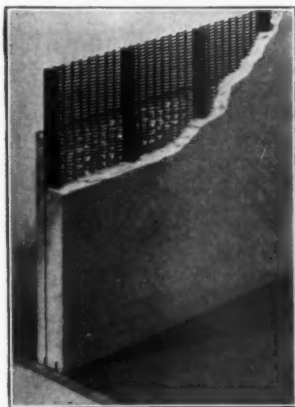
Milcor \frac{3}{4} " Stay Rib Lath No. 3 used with ribs perpendicular to floor, no upright channels required. This is a Milcor innovation. Runner channels only are needed at the floor and ceiling for alignment. Write for full particulars.
