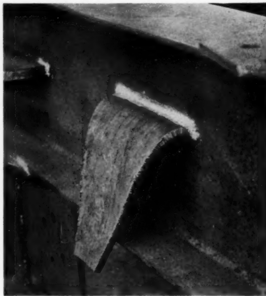
AT LEFT: DETAIL OF END OF 3'-6" x 35' BUILT UP SHOP WELDED GIRDER USED FOR A LARGE CRANE RUNWAY. AT RIGHT: TEST OF A WELDED JOINT MADE BY WELDING A 13" x 10" x \frac{3}{8} " PLATE ON EDGE TO THE WEB OF AN I-BEAM. PLATE BENT AS SHOWN BY SIXTY BLOWS WITH A TWELVE POUND SLEDGE HAMMER. A SIX HUNDRED POUND STEEL RAM HUNG FROM AN OVERHEAD CRANE AND OPERATED BY FOUR MEN DIRECTED FORTY-SIX BLOWS AGAINST THE WELDED PLATE CLOSE TO THE WELD
