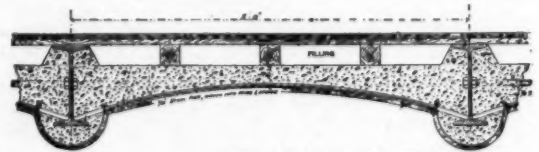
System A—Type 2. Warehouse Construction, with Sleepers
