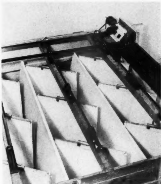
Position of louvres at mid-forenoon, view looking west, with louvres H in normal position and louvres V rotated normal to the sun
