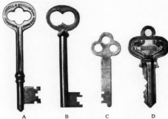
TYPES OF KEYS IN COMMON USE TODAY. A. ROUND KEY WITH SOLID CYLINDRICAL SHANK AND STEM, WITH WING BIT. B. BARREL KEY, WITH A TUBULAR STEM. C. ORIGINAL TYPE OF FLAT KEY FOR CYLINDER LOCKS. D. PARACENTRIC KEY, THE LATEST AND BEST KIND OF FLAT KEY, ALMOST UNIVERSALLY USED FOR EVERY VARIETY OF CYLINDER LOCK
