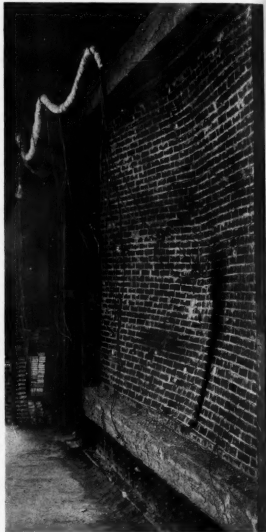
Fig. 9. U exposed side of a 4" restrained shale brick wall 3 hours after start of fire test, Test No. 13
