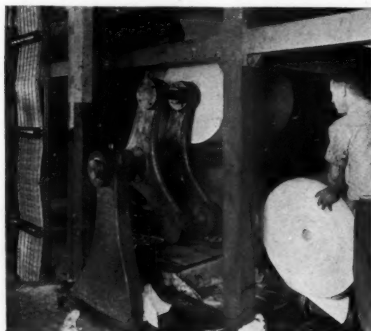
Loading the newsprint reel on second floor from which the newsprint is fed to the presses on the floor above. Dispatch conveyor at left
