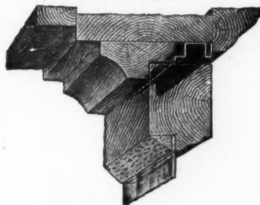
Cross-section through sash and window frame at top, showing installation of AiR-Way track and the tight application of sash.
