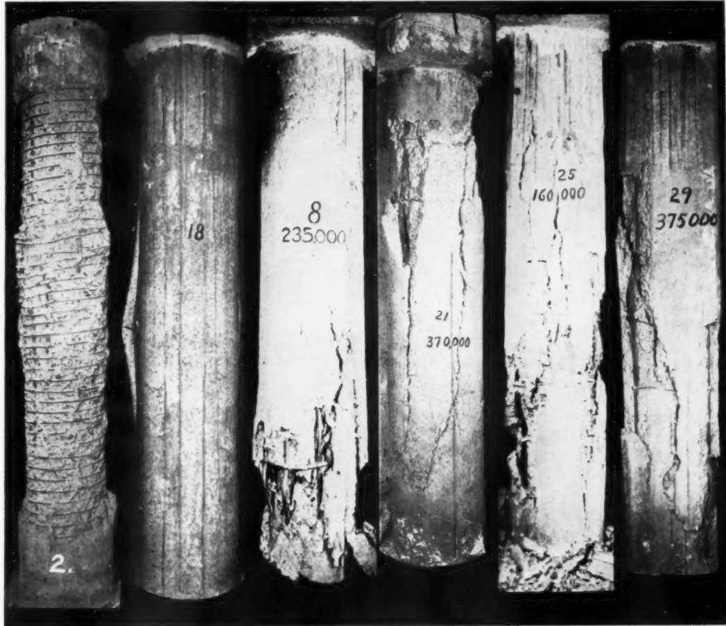
Col. 2 Col. 18 Col. 8 Col. 21 Col. 25 Col. 29 Gravel concrete failed in 4 hr. 15 min. Concrete came off early in test. Limestone concrete. After 600,000 lb. at end of 4 hr. fire test. Gravel concrete. Round. Limestone concrete. Round. Gravel concrete. Square. Limestone concrete. Square.
